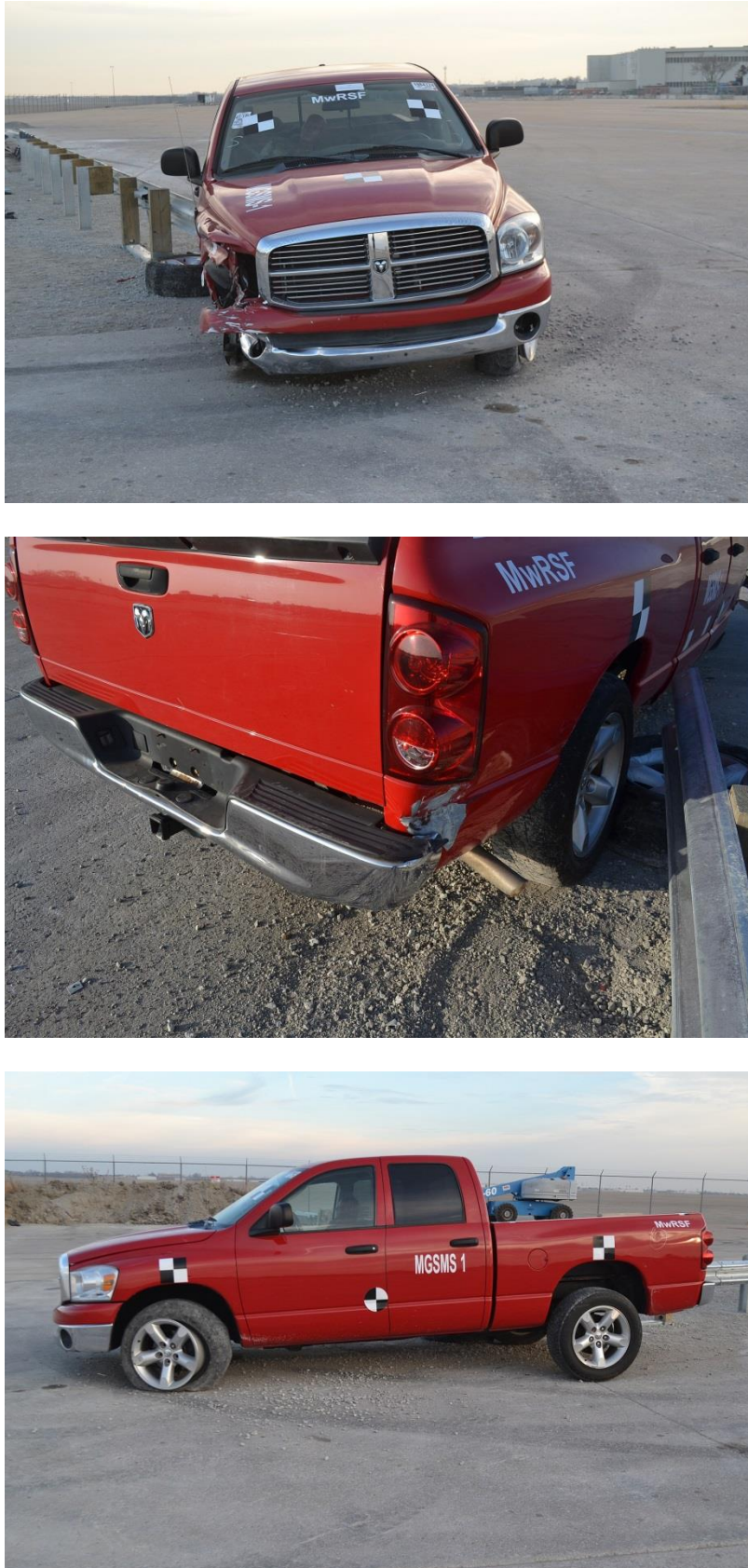
Figure 90. Vehicle Damage, Test No. MGSMS-1
