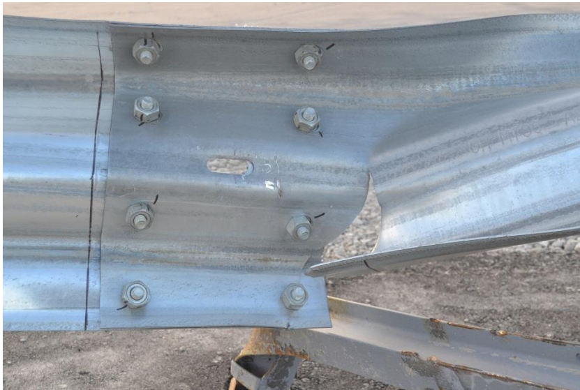
Figure 88. System Damage – Rail Tearing, Test No. MGSMS-1
