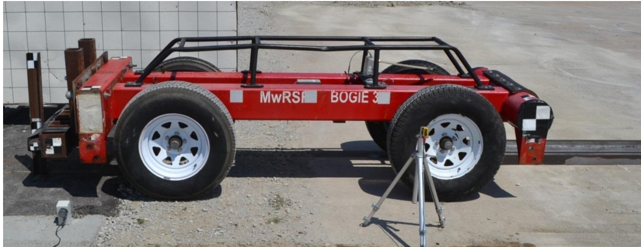
Figure 3. Rigid-Frame Bogie on Guidance Track
