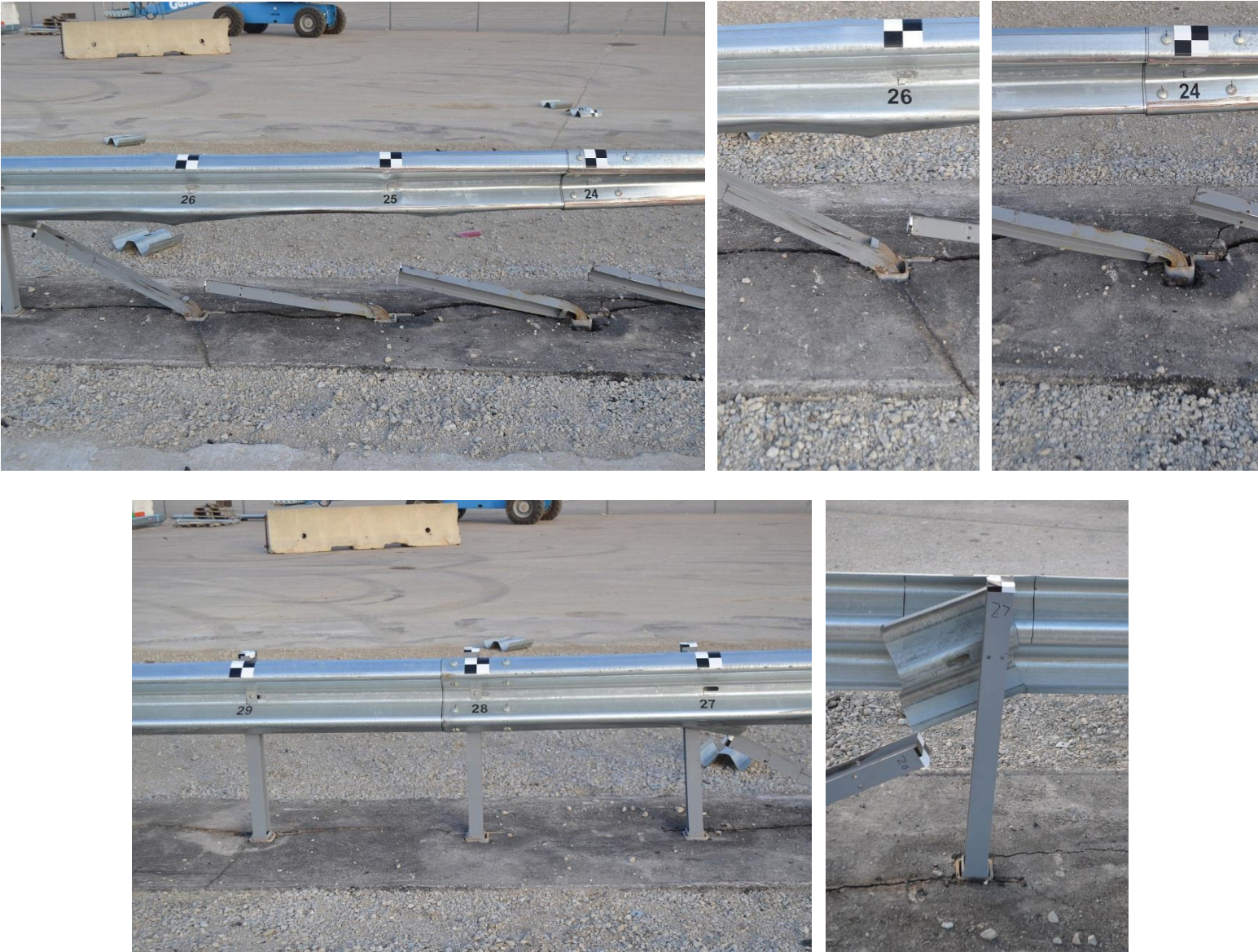
Figure 86. System Damage – Post Nos. 24 Through 29, Test No. MGSMS-1
