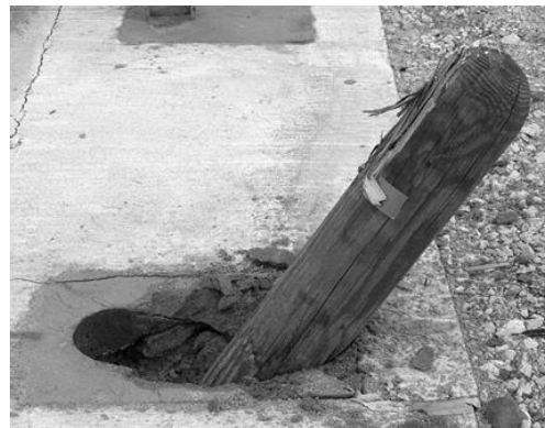
Figure 1. Pre- and Post-Test Photos of Posts in Grout-Filled Leave-Outs [3]
