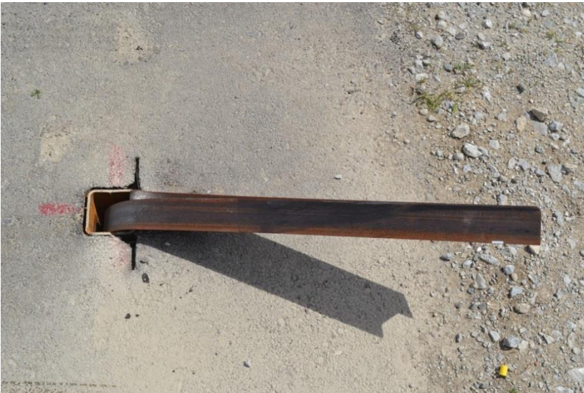
Figure 31. Pre- and Post-Impact Photographs, Test No. MSSP-1
