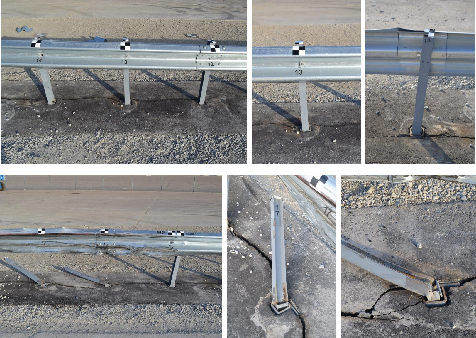
Figure 83. System Damage – Post Nos. 12 Through 17, Test No. MGSMS-1
