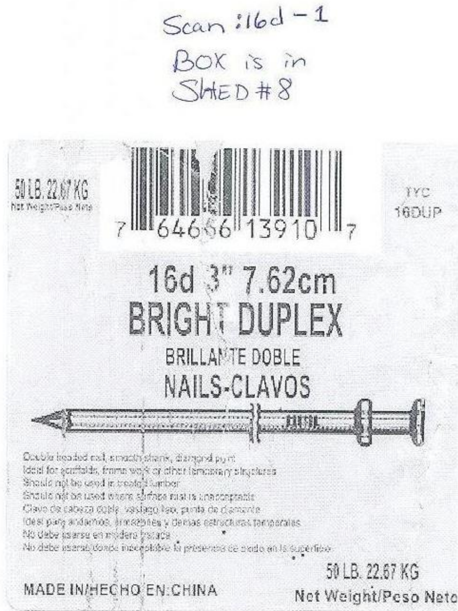
Figure C-3. 16D Blockout Nail Material Specification, Test No. MGSMS-1
