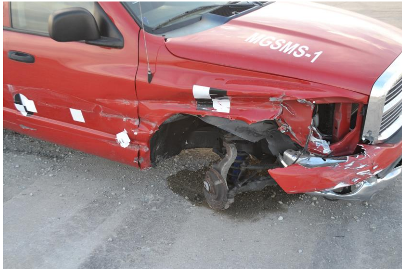
Figure 89. Vehicle Damage, Test No. MGSMS-1
