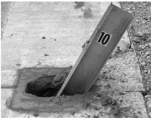
Figure 1. Pre- and Post-Test Photos of Posts in Grout-Filled Leave-Outs [3]
