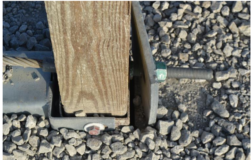
Figure 87. System Damage – Asphalt Fracture and Anchor Movement, Test No. MGSMS-1
